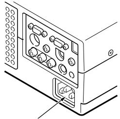
Connect the AC power supply cord (supplied) to the projector.
